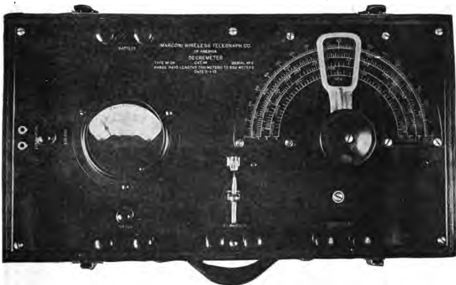
Fig. 220—The American Marconi Company's Decrometer.
